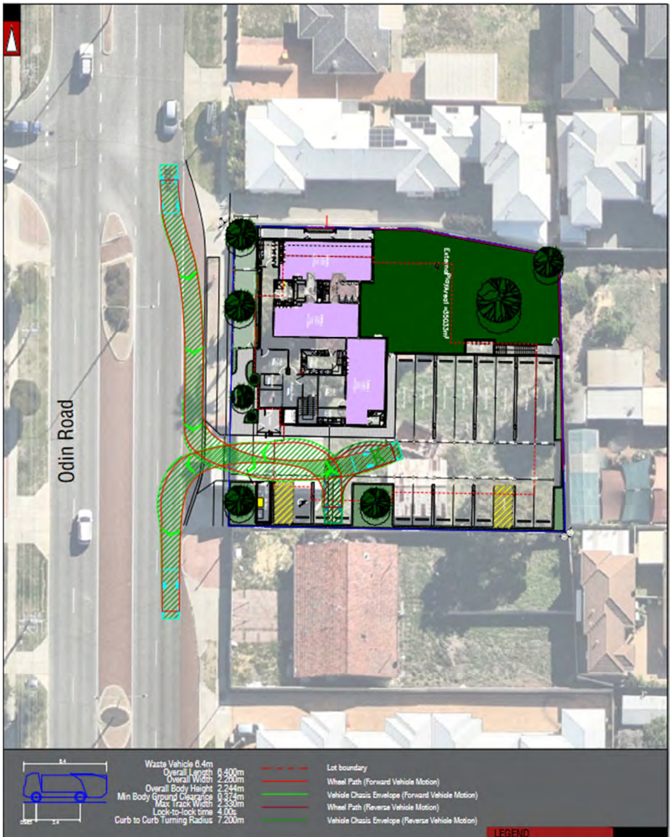
Figure 3 – On-site turning area for the waste collection truck (KCTT)
