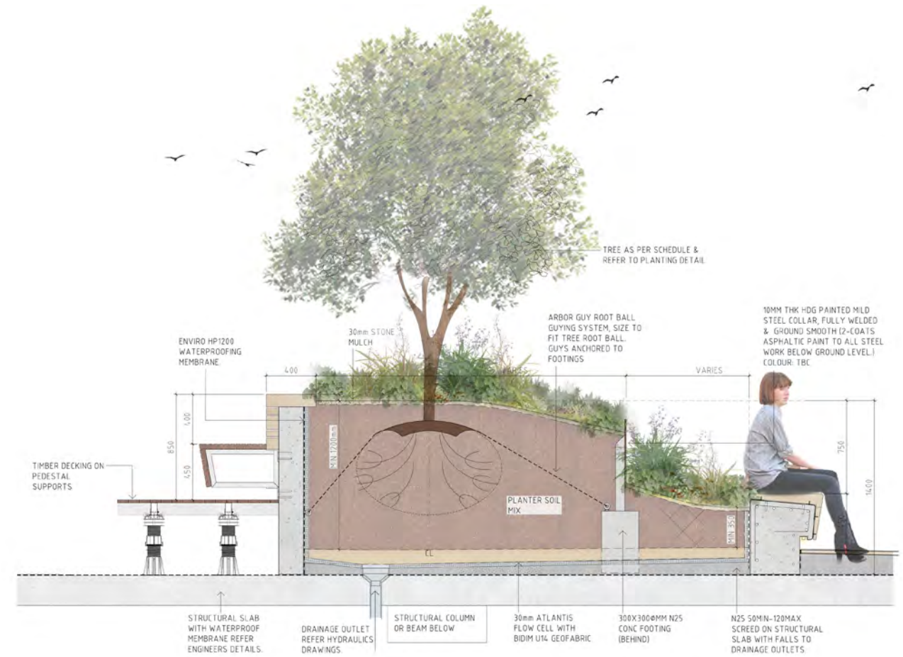
02 PLANTER ON STRUCTURE WITH SEATING AND STEEL EDGE
