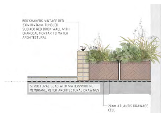
03 MASONRY WALL WITH HDPE PLANTER INSERTS
