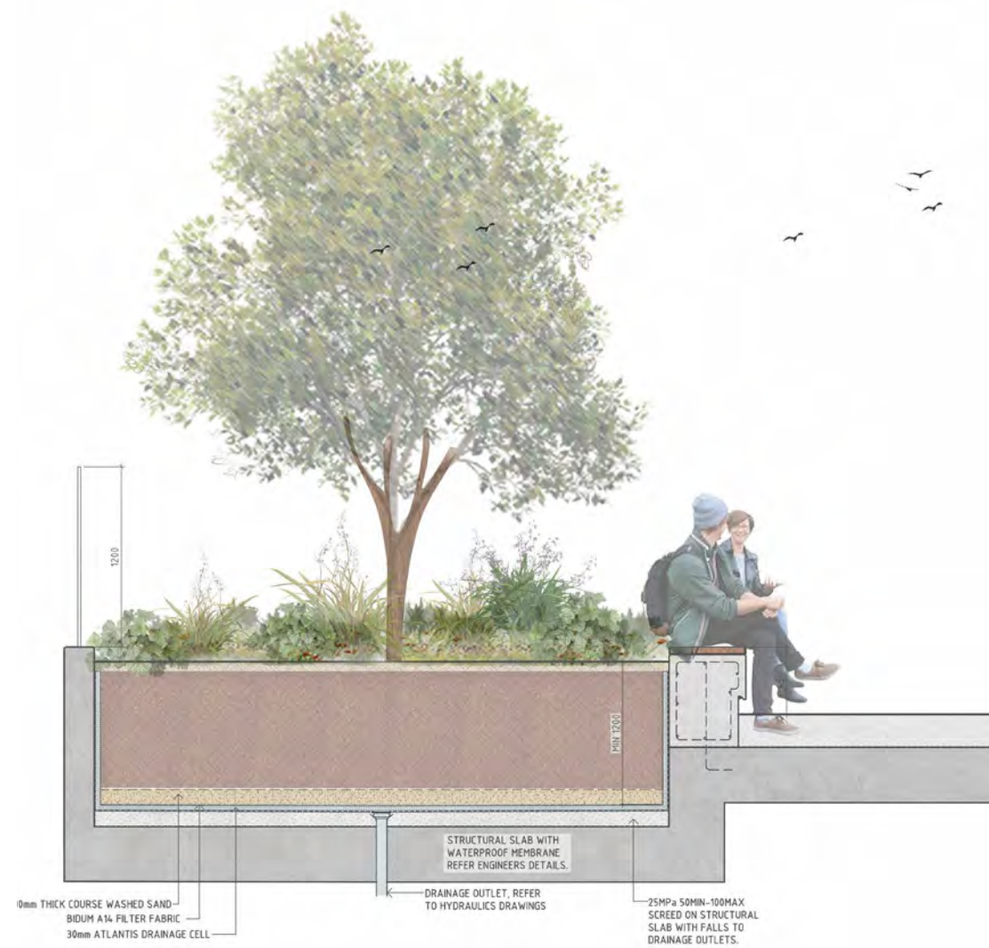
01 PLANTER ON STRUCTURE WITH SLAB SET(DOWN AND SEATING
