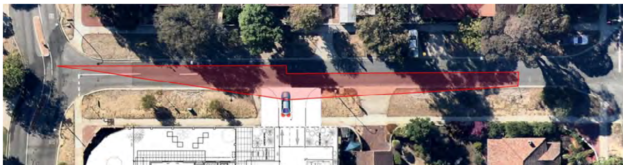
Figure 7 – Clear 45 m sight distance to and from access driveway
