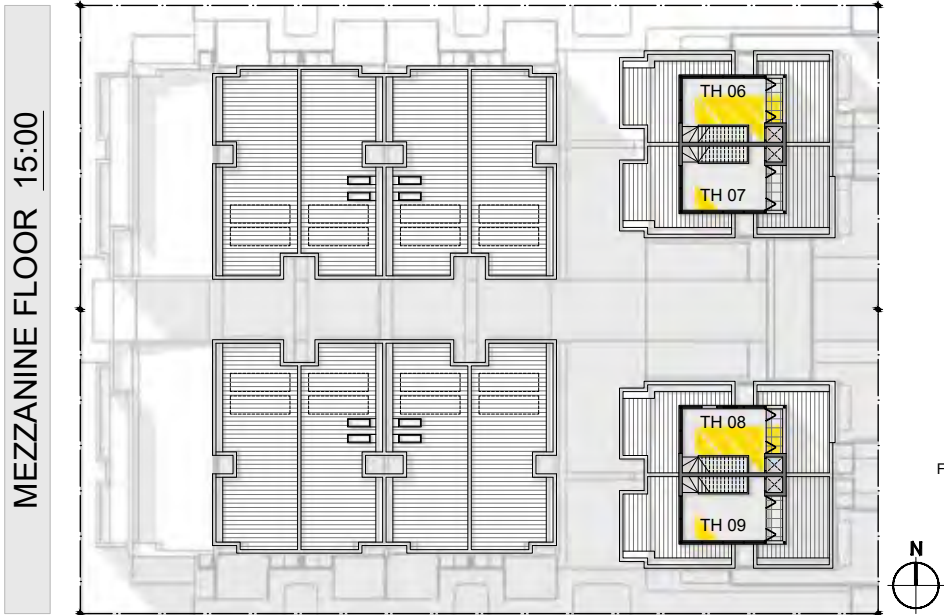
Figure 4.1b The hours of sunlight that can be expected in mid winter are directly related to the orientation of the windows or balconies. To achieve 2 hours sunlight (refer A4.1.1(a)), windows must be facing between west and north; or between north and east. This diagram shows the optimal orientation for sunlight to reach any portion of a window or balcony on 21 June in climate zones 4, 5 and 6.
