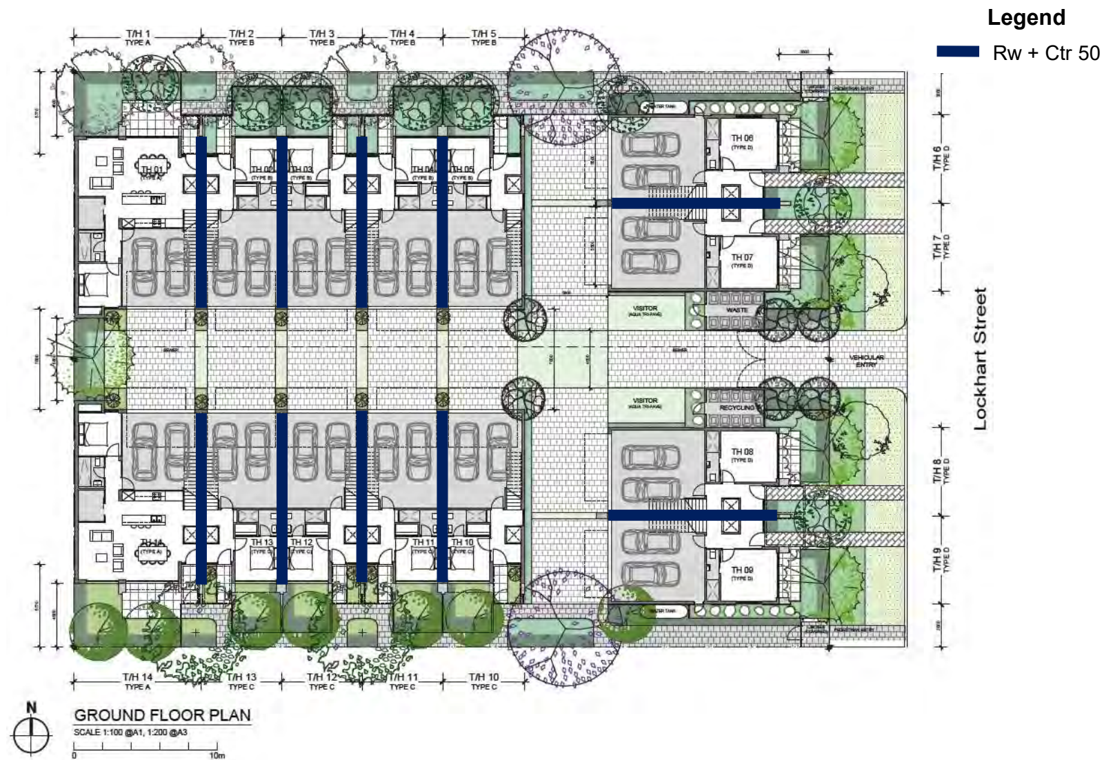
Figure 6: Party walls for the ground floor.
