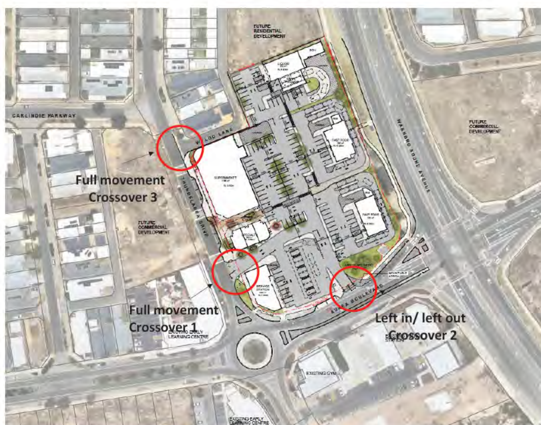
Figure 2. Proposed access/egress system
