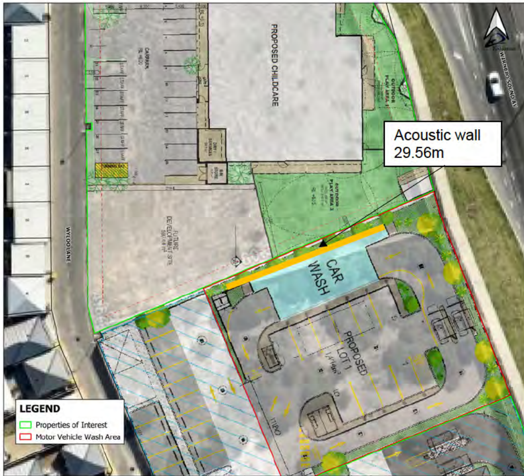
Figure 6. Extent of Acoustic Wall to Northern aspect
