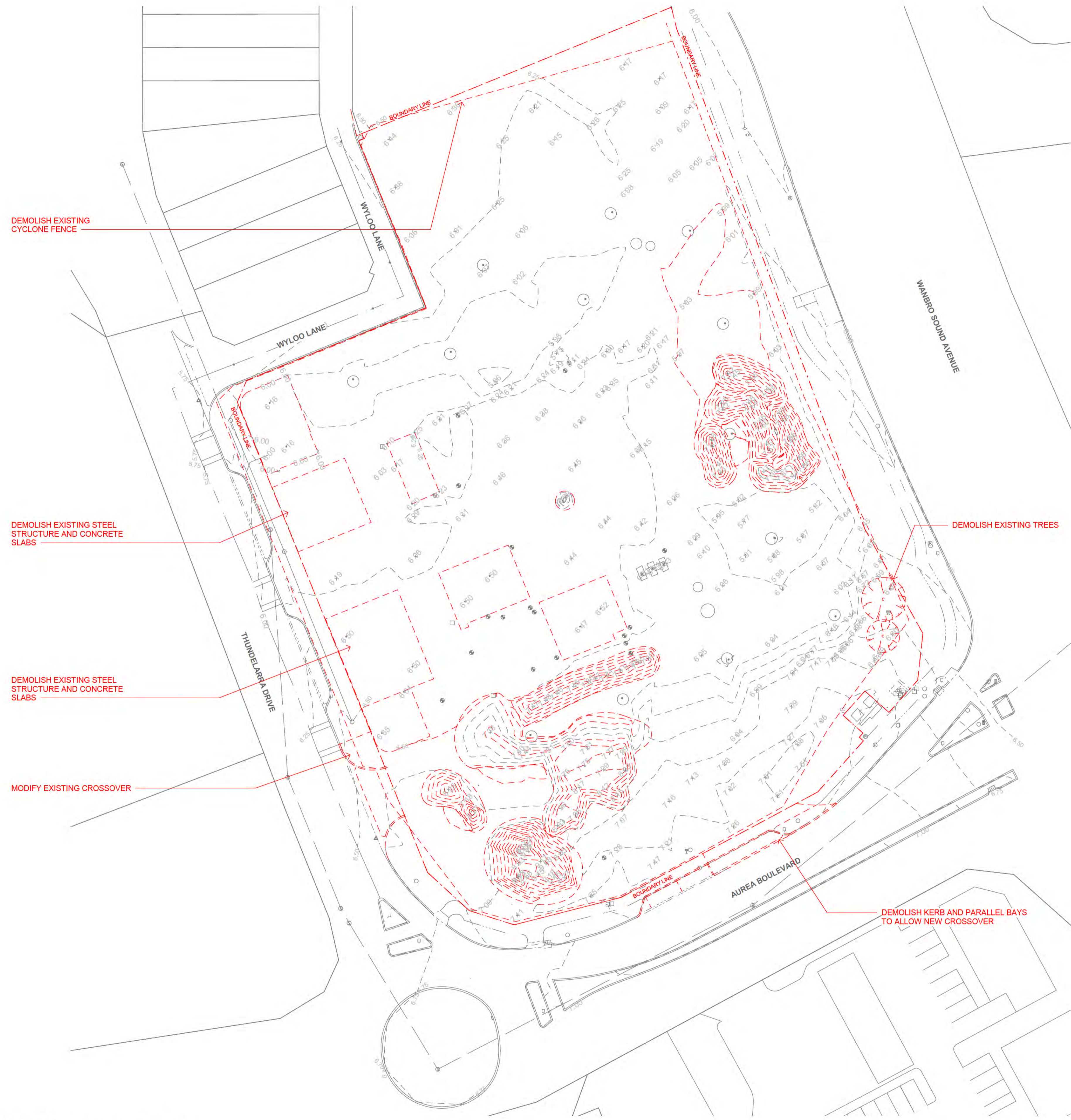
1 PROPOSED DEMOLITION PLAN 1:400
