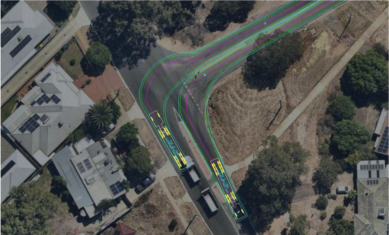
Figure 4-2: Swept path 19m semi-trailer, Stirling Crescent to Bushmead Road
