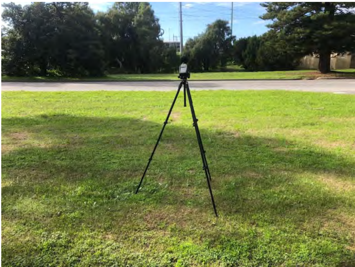
Figure 3-1: Photograph of Sound Level Meter on Site
