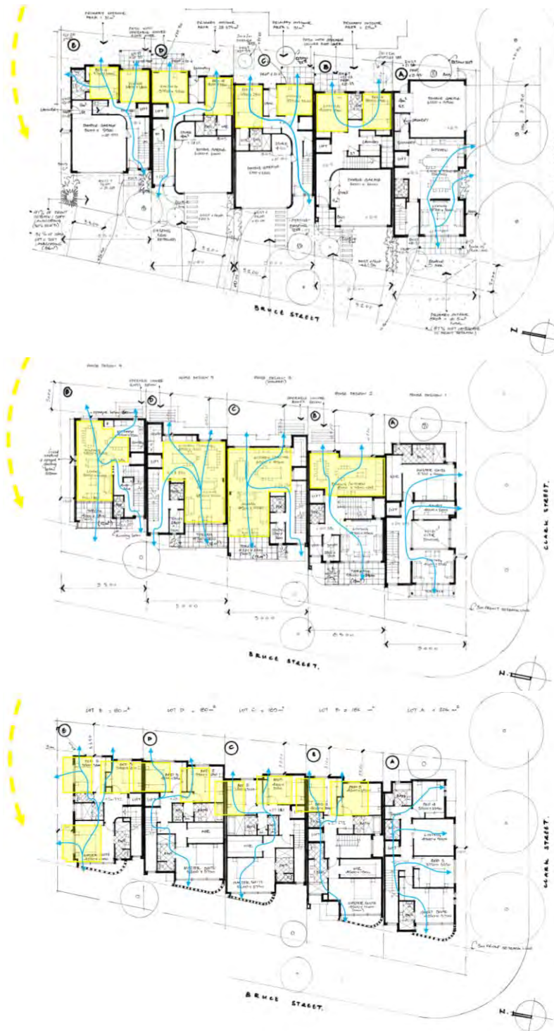
Figure 2: Cross Ventilation of all Primary Living Areas
