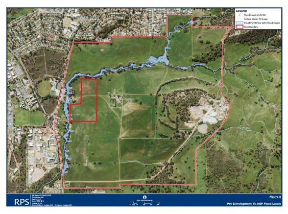
Figure 1: Pre-development surface water features and flood extent
