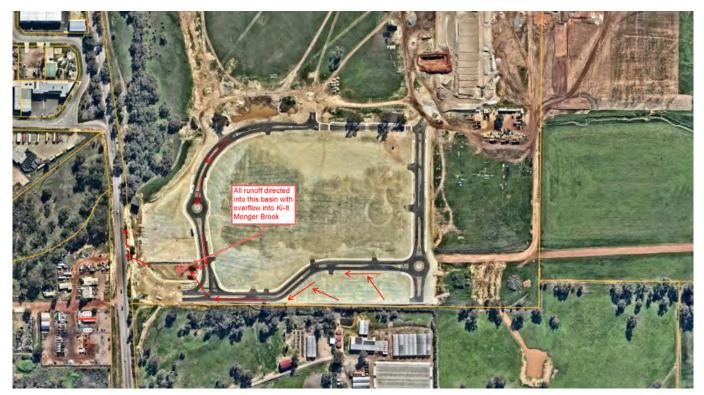
FIGURE 7: Stormwater Drainage Area
