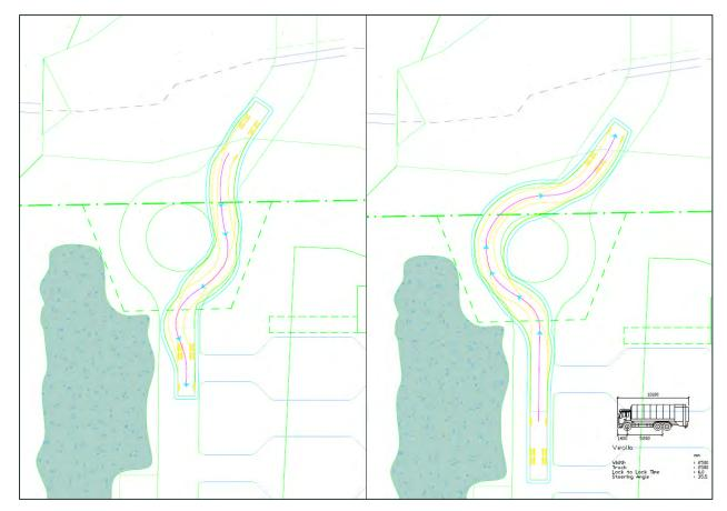
Figure 4 Swept Path - Waste Vehicle Collection (Entry Gate)
