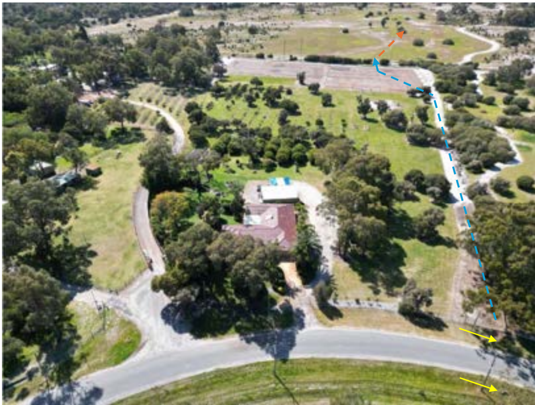
Plate 10: Aerial view. Drain within site near eastern boundary no longer exist following earthworks in early 2000s. Yellow arrows show culvert under road, blue arrow shows the previous drain pathway, and orange arrow shows the still existing drain located downstream of the site. Source of Image: Galt Geotechnics WAG240411-01 001 R Rev0.
